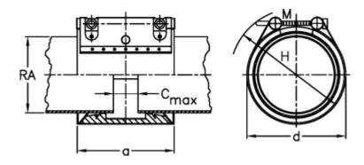
a = 142 C max with insertion band = 35 d = 285 H = 315
